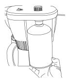
2a - For use with Butane open the fuel compartment remove the included brass butane adaptor, thread the adaptor onto a butane canister and insert a the butane canister and adaptor and attach by pushing up and turning counter clockwise.
